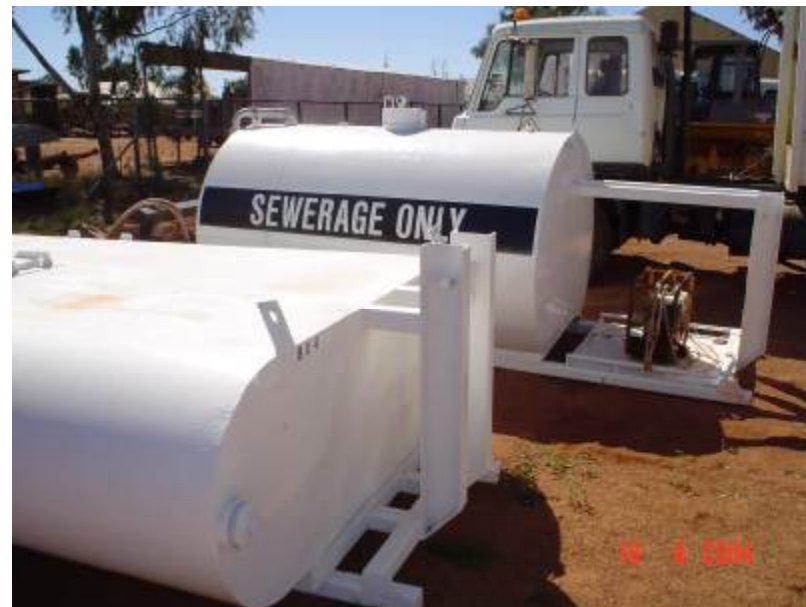
The water tank, sewerage tank and diesel tank have been converted for use with the demountable system by the customer.
