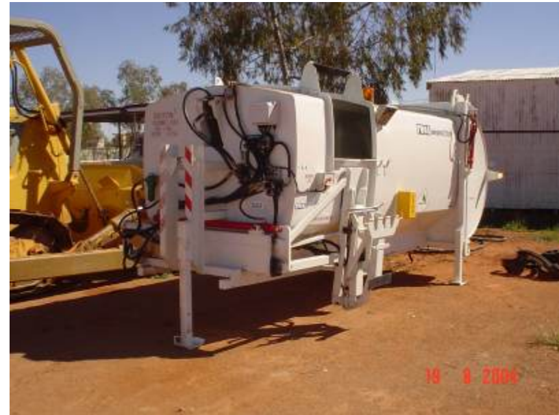
The water tank, sewerage tank and diesel tank have been converted for use with the demountable system by the customer.
