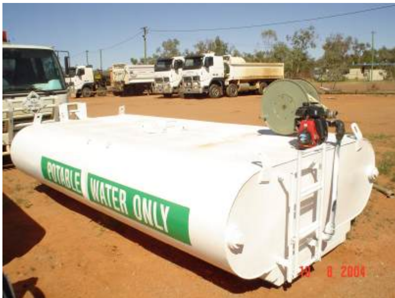
The water tank, sewerage tank and diesel tank have been converted for use with the demountable system by the customer.
