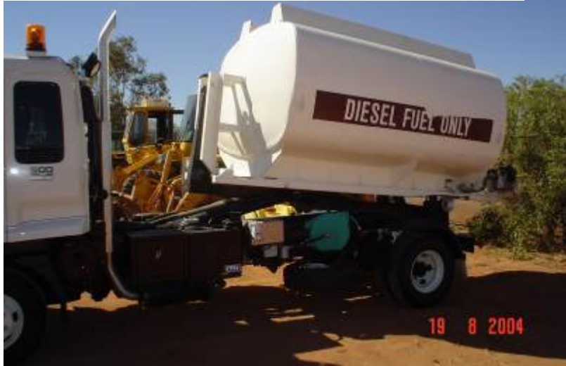
The water tank, sewerage tank and diesel tank have been converted for use with the demountable system by the customer.
